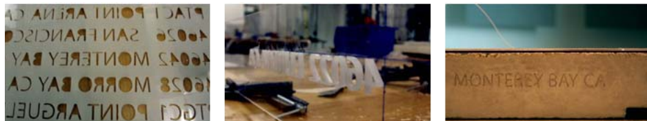
Figure 71. Laser cutting for labeling
