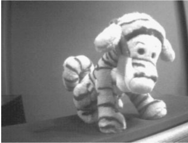
Fig. 7.6.8. MIT Media Lab Affective Computing Group, The Affective Tigger reacts to his playmate with a display of emotion, based on his perception of the mood of play.
