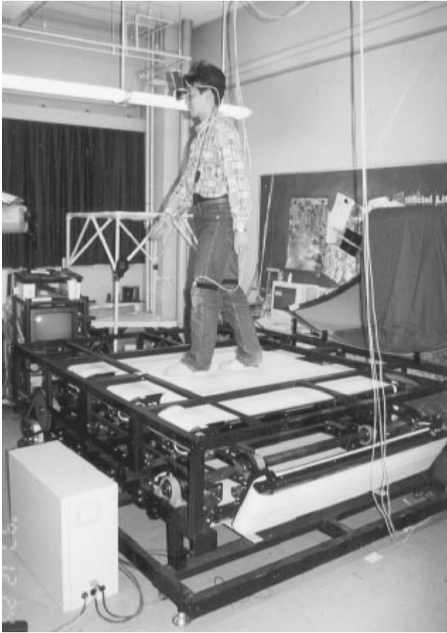
Fig. 7.1.9. Hiroo Iwata, Virtual Reality Laboratory, University of Tsukuba. Infinite Plane —a computer-controllable walking plane that can read and respond to a walker's action, ( http://intron.kz.tsukuba.ac.jp/index.html ).
